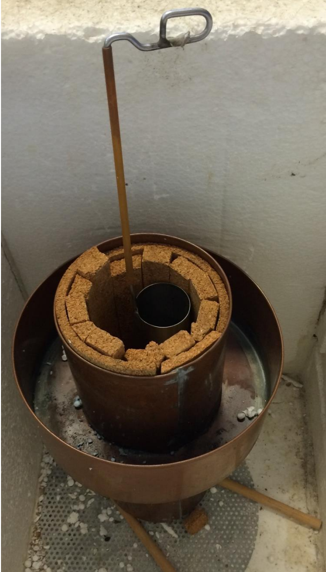
Figure 2.1 Copper slow cooling chamber for preparation of fungal strains for cryopreservation.
